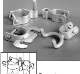
The gravity type self closing hinge set has no springs to wear out. By raising the bottom hinge set you can increase the force at which the gate will close.
