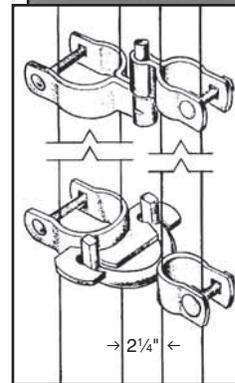
The gravity type self closing hinge set has no springs to wear out. By raising the bottom hinge set you can increase the force at which the gate will close.
