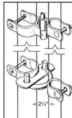
The hinges can also be used to compensate for slight grade changes making it possible to install the gate on a hill, yet keep the bottom of the gate close to the ground.
